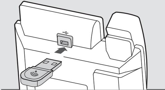
Insert the Wi-Fi USB Dongle into the USB port on the back of the phone.
