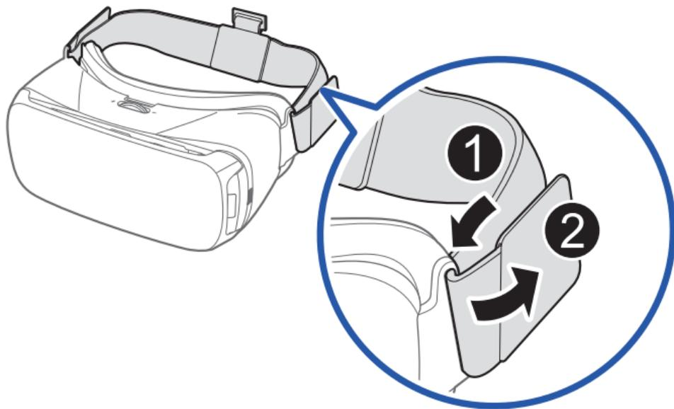
3. Carefully insert the hook (from the top head strap) into the front bar of the Gear VR (1), then pull it upward until it locks in place (2). The hook snaps when secured.
