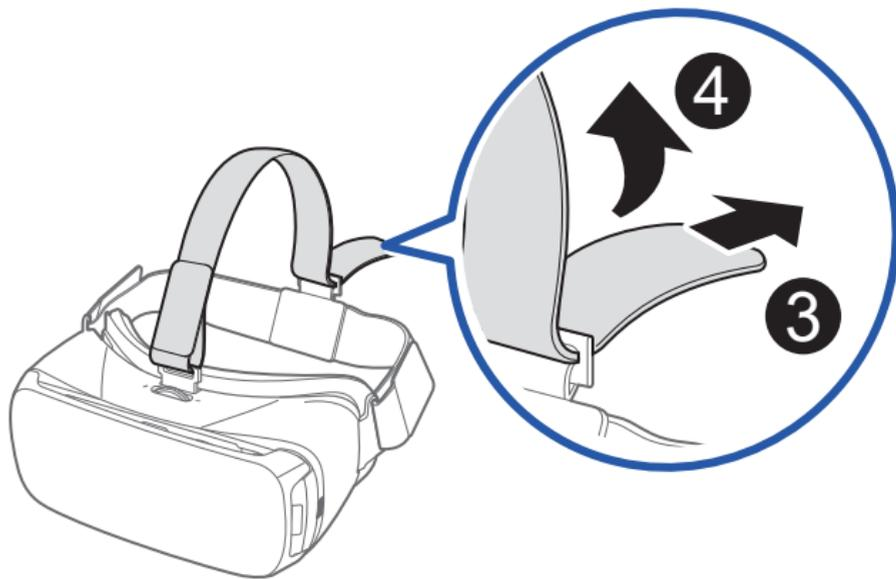
**Note:** The head strap contains a longer velcro strip and is used to secure the front of the Gear VR frame.
