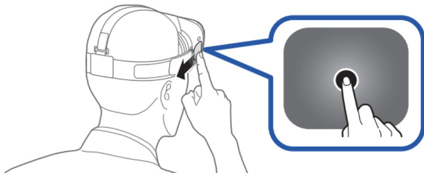
**Note:** When you are not wearing the Gear VR, the touchpad does not work
