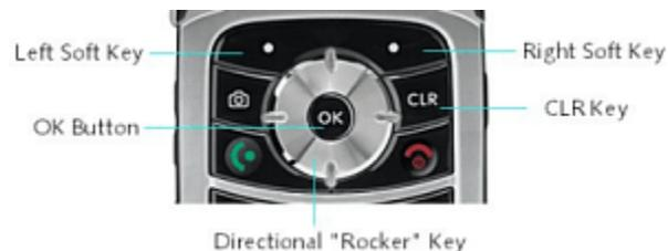
The Left Soft Key (LSK), Right Soft Key (RSK) and OK button vary in function depending on what you are doing. The bottom of the screen displays their current function, as shown in the illustration, right: LSK on the left, RSK on the right, and OK button in the middle. In this example, the LSK sorts a list, the RSK displays a list of options, and the OK button begins navigation to the selected location.
